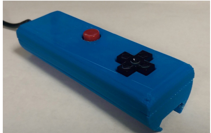
Figure 3: 3-D Printed Prototype FWS-I Remote Switch
